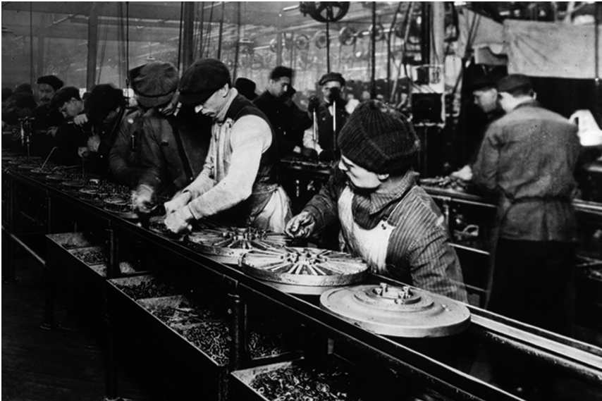
Figure 1.3 T Model Ford Flywheel magnetos for the T Model Ford on a moving production conveyor belt at Highland Park Michigan Plant USA. This was the first use of a moving conveyor belt production and assembly.
